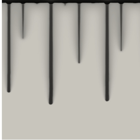
Figure 6: A solution of the two-dimensional system corresponding to (1.1)–(1.2) with play-type hysteresis and \tau > 0 , for the setting see [14]. In this result, the fingers are of moderate length and the drainage process in the fingers has not set in. This justifies the assumption that only imbibition and scanning curves are relevant.
